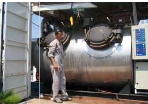
Treating medical waste in situ – thanks to the LIFE mobile sterilisation plant
