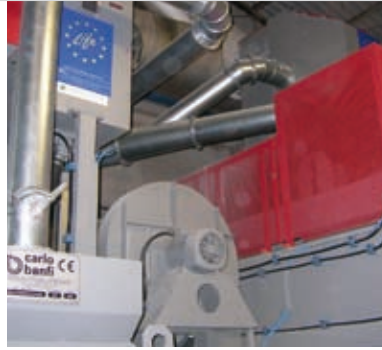
The microfinishing spraying technique replaced highly polluting grinding and polishing stages in the ceramic tile production process
