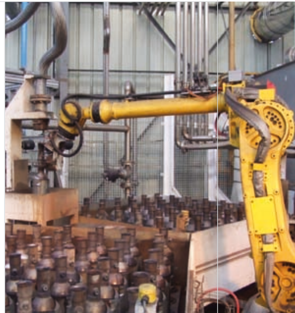
Dunking and washing of the particulate filters
