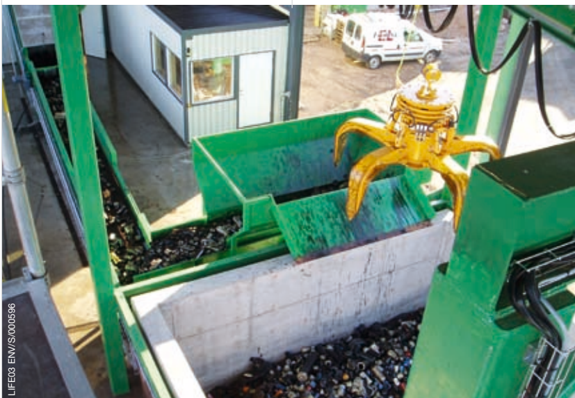
Bunker to receive used vehicle oil filters and conveyer belt
