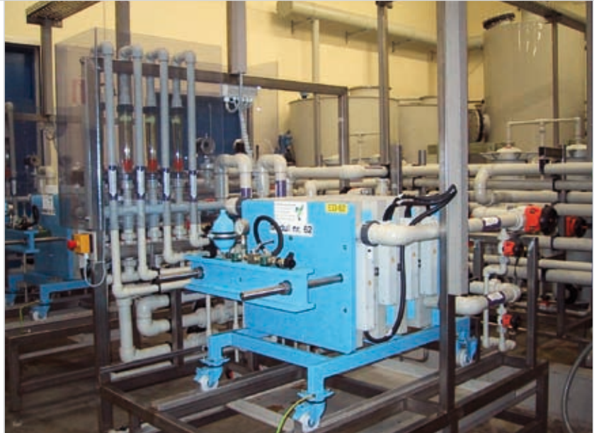
Membrane modules are the vital parts in the electrodiolysis process.
