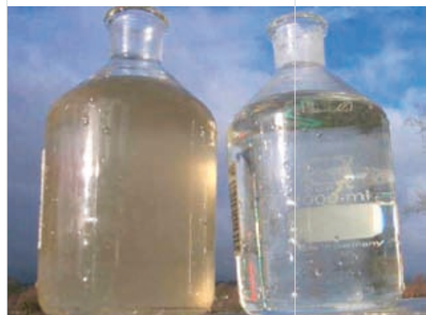
Before and after AFM treatment of sewage effluent
