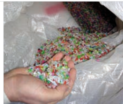
WPC can make use of more than just a handful of recycled pellets from thermoplastic waste
