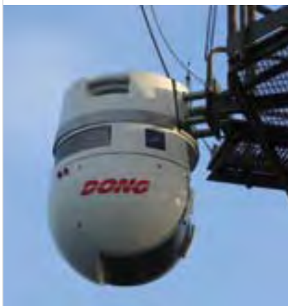
Close-up of the permanently-mounted OSIS sensor
