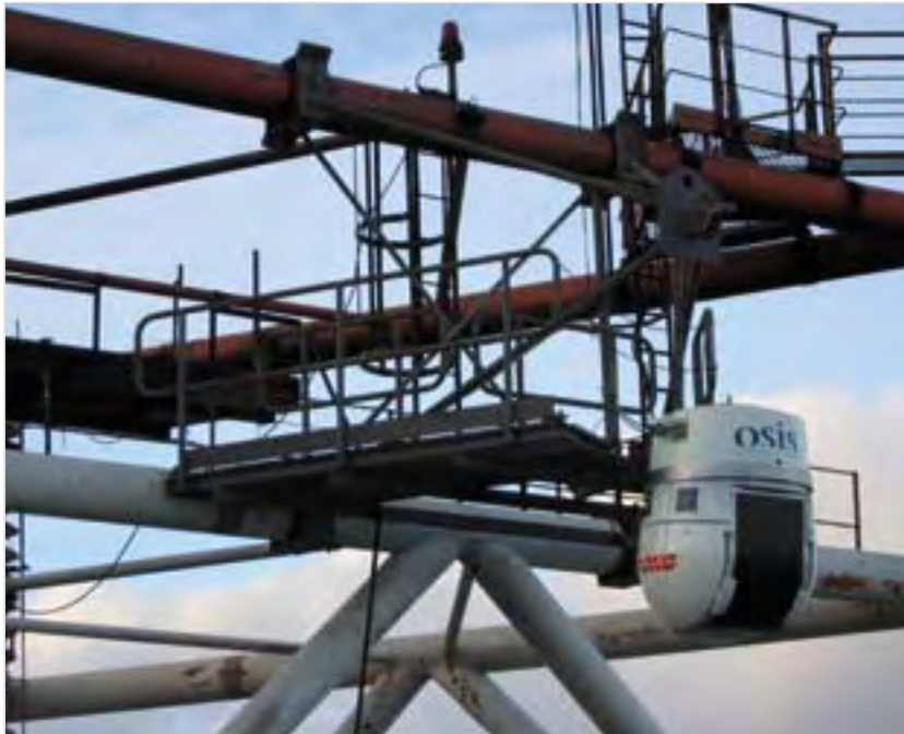
'Real-time' OSIS sensor at the front of an oil rig
