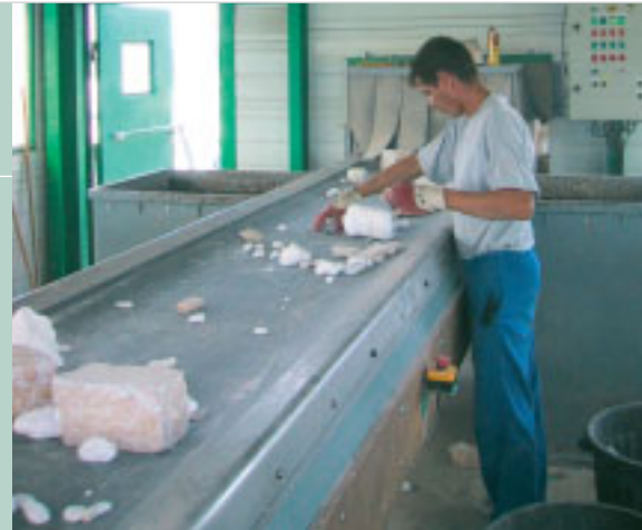
Waste residues are sorted on this conveyor belt – helping to identify the material that can be recycled
