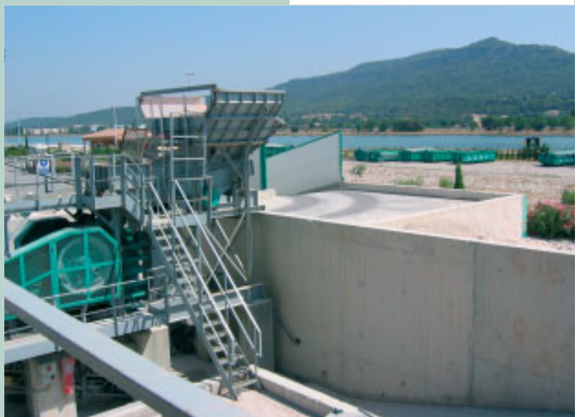
Valoref's Bollène industrial site in France: waste is first broken up to a suitable size for the sorting process.
