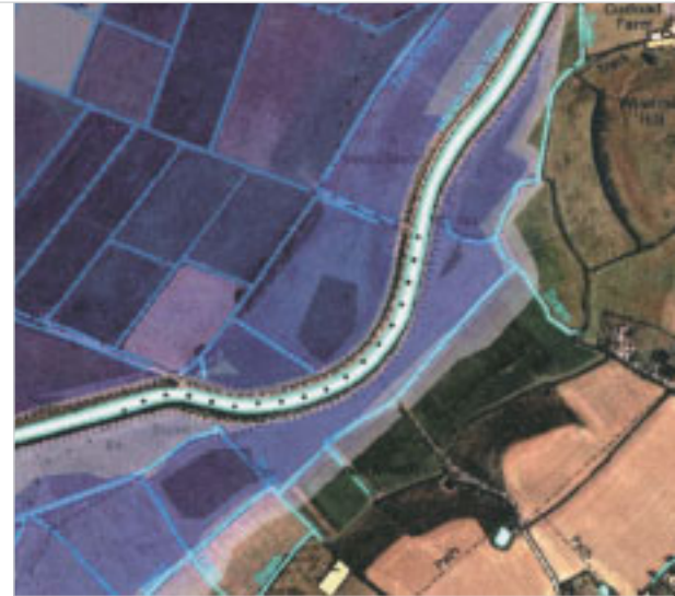
Flood simulation using hydrological modelling and visualised through GIS technology.
