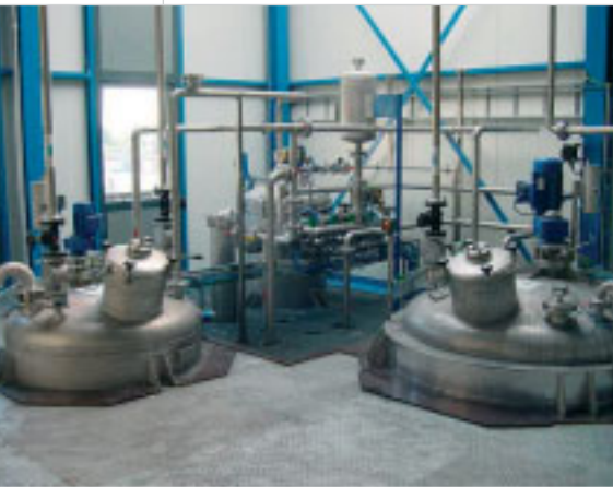
The installation of the filtration unit (shown here) made it possible to re-use the spent rinsing MMA twice before sending it to distillation. This resulted in a 50% reduction of the waste stream.
