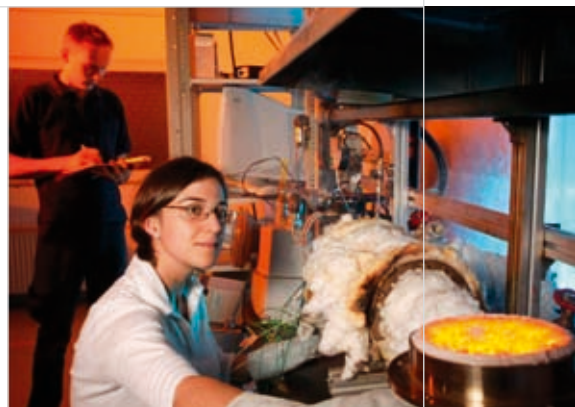
The project team produced a modulating oil burner of small capacity that can be adapted to an oil-condensing boiler.
