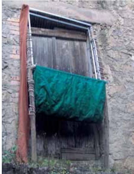
Figure 4.4 - A harp-trap set near a bat roost exit. Flying bats hit the nylon threads and fall into the bag, from which they can be easily removed (Photo by G. Maglio).
