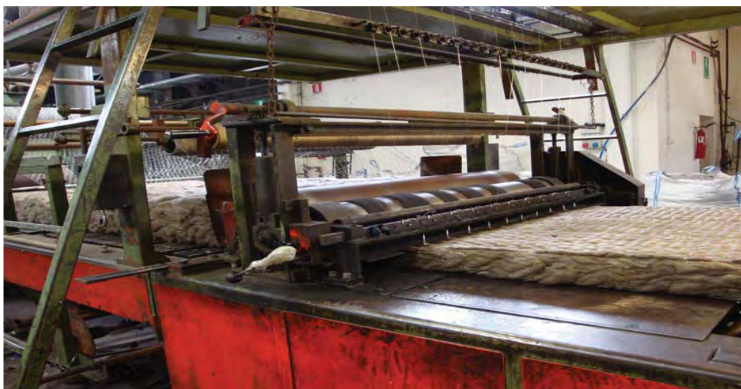
Figure 3 - Rock wool production from bottom ash and fly ash
