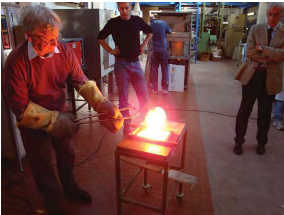
Figure 2 - Laboratory-scale glass production for rock wool
