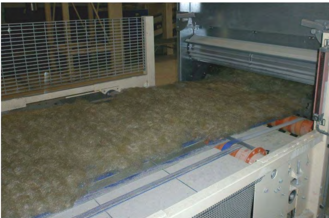
Figure 9 - Rock wool mat forming
