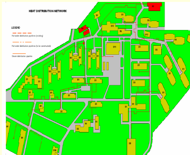
Figure 6. Student City, Centre-boiler houses and Heat-network
