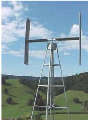
**Figura 3-43 Turbina Darrieus ad H**
